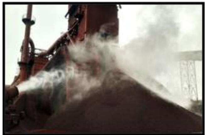
Photographs of dry fog system and fog cannon installed at transfer point
