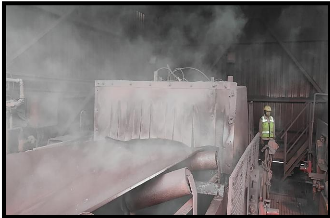
Photographs of dry fog system and fog cannon installed at transfer point
