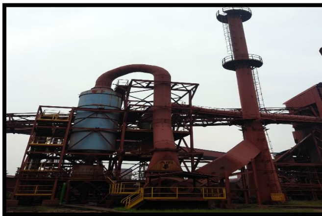
Photographs of Electrostatic precipitator and Wet scrubber installed to capture for Dust generated from process
